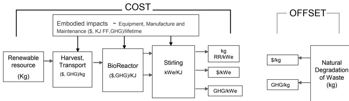
**Figure 1. Biogas/Stirling life-cycle model**
